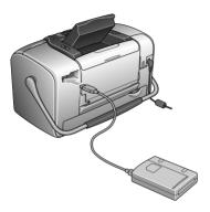
□ For a flash memory drive, plug it into the EXT/IF port on the back of PictureMate.
